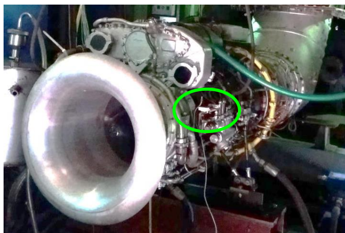
Fig. 9 – Vibrations harnessing on a Klimov TV2-117A gas turbine turboshaft engine
