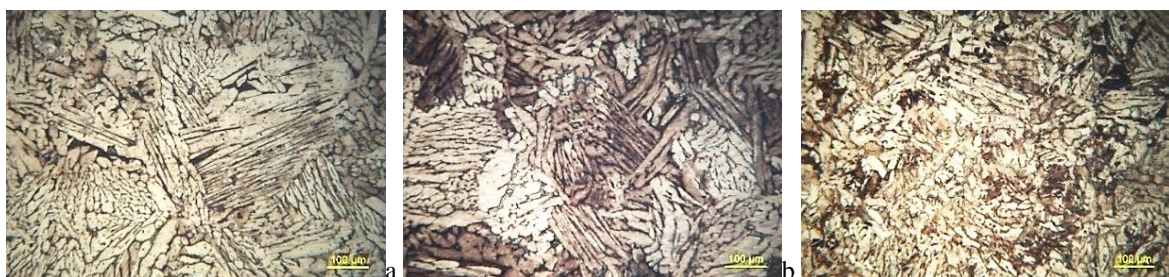
Fig. 3 Optic microscopy with ADAM 17-4 PH alloy microstructure: a) as printed state; b) material after treatment 1; c) material after treatment 2
